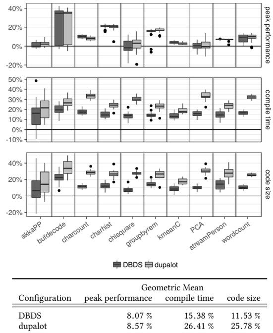
Figure 7. Java/Scala Micro Benchmarks; peak performance (higher is better), compile time (lower is better), code size (lower is better).
