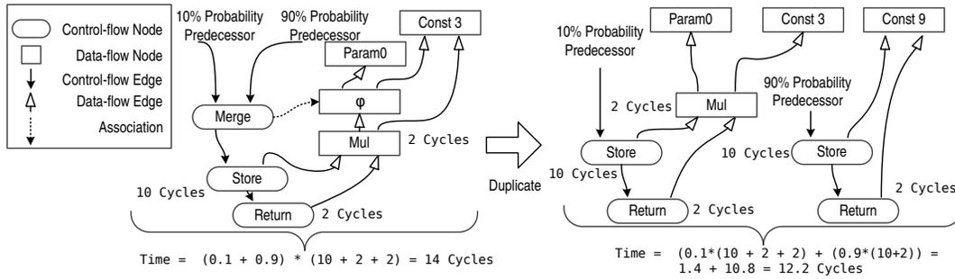
Figure 4. Node cost model example.
