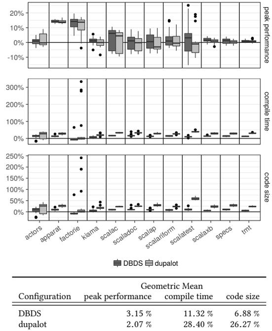
Figure 6. Duplication Scala DaCapo; peak performance (higher is better), compile time (lower is better), code size (lower is better).
