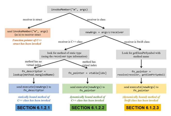
Figure 6.5: Processing of invokeMember messages in Sulong
