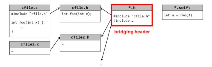
Figure 3.4: Principle and concept of Swift-C/C++ interoperability
